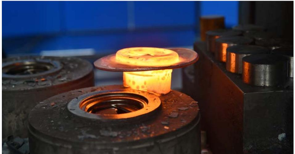
mind for investigations in the future. The experimental trials with the realized force-closure tools revealed, that the punch drive at insertion and extraction requires high forces. Especially extracting the punches causes forces  $> 20$  kN, which must be already considered at the stage of designing, so the tools are able to endure these forces.
